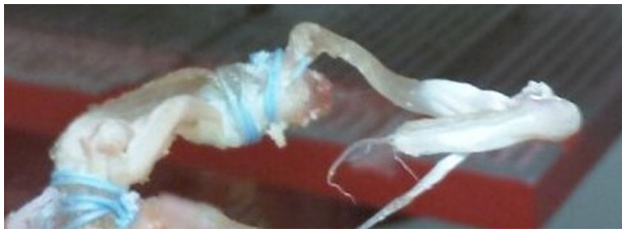
Fig. 5 Mode of failure: tendon slippage across the suture (“quadrupled” configuration)
