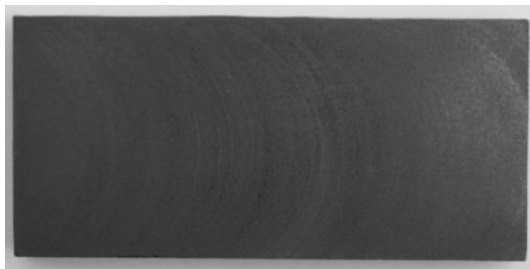
Figure 4 Photograph of SiC ceramic workpiece machined by the compound process (130 mm × 60 mm).
