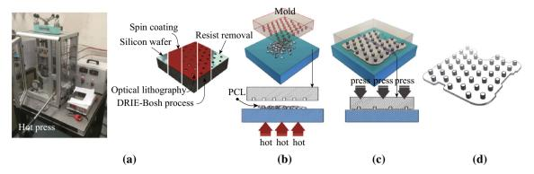
Fig. 2 Schematization of the fabrication process for 3D PCL pillared scaffolds using a hot press (on the *left*). a Silicon master production. b Micromolding melting step. c Micromolding pressing step. d Final structure obtained after solidification and detachment. Figure adapted from [17]
