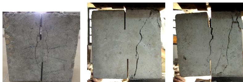
Fig. 5 Crack patterns in different mode II specimens under various test setups. a DNC specimens. b 4PS specimens. c BND specimens. d ENP specimens.
