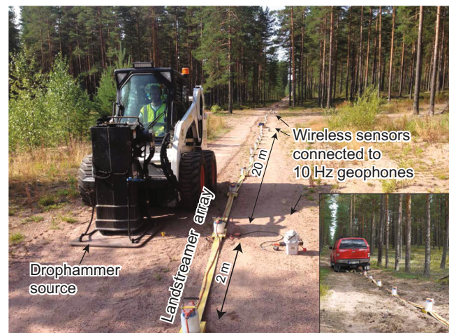
Fig. 6 Field conditions during the seismic survey (July 2014). Bobcat mounted drop-hammer (500 kg) was used to generate seismic energy at every shot location (only fired close to the streamer sensors). Inset shows a photo of the streamer while moving to a new position in a forest track with uneven and loose sediments along part of profile 2. The wireless recorders (10–20 m apart) connected to 10 Hz geophones were spaced along the landstreamer array and fixed for the whole profile. Photos by Alireza Malehmir
