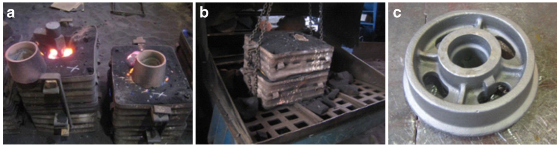
Fig. 1 The view of the moulds after casting (a), prepared for the crushing (b) and the casting (c)
