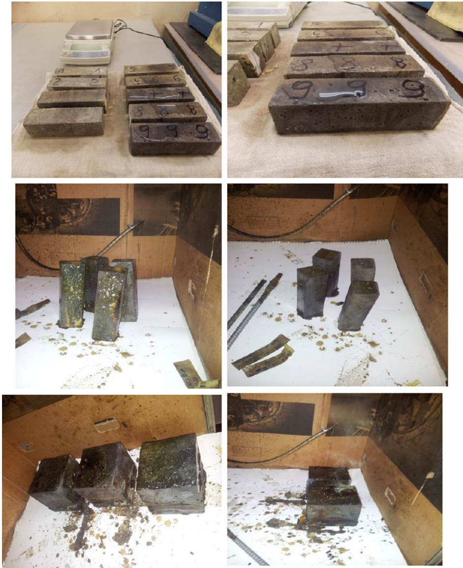
Fig. 2 View cement composites impregnated with the waste of sulfur
