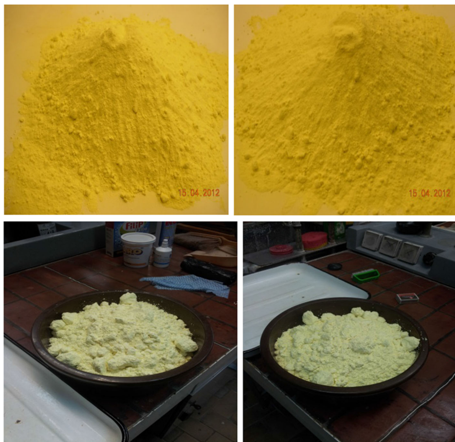
Fig. 5 View of the sulfuric binder used in the investigations
