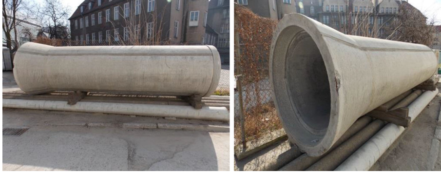
Fig. 8 View of the city collector impregnated with special polymerized sulfur
