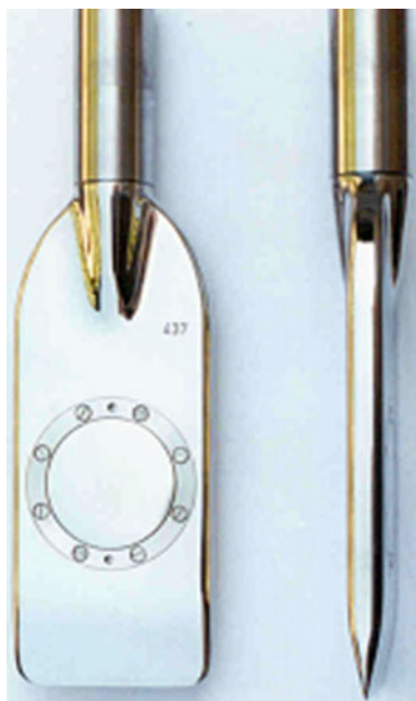
Fig. 2 The flat dilatometer—front and side view (from Marchetti et al. [7])
