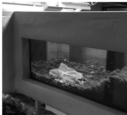
section (left photograph), this shelter was used by all except one trout. A net placed over the wood bundle simulated the effect of shelter exclusion by anchor ice (right photograph)
