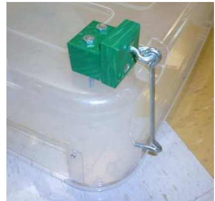
Figure 31: Hook used to attach Retriever to base cart
