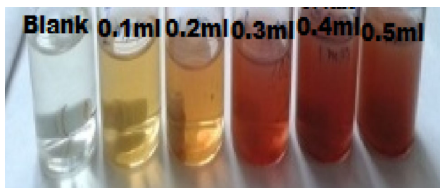
Fig. 2 Ag nanocolloid samples (colour changes with changes in concentration of leaf extract)
