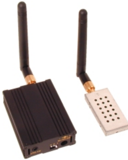
Figure 4-11 Black Widow 2.4 GHz audio/video transmitter and receiver.
