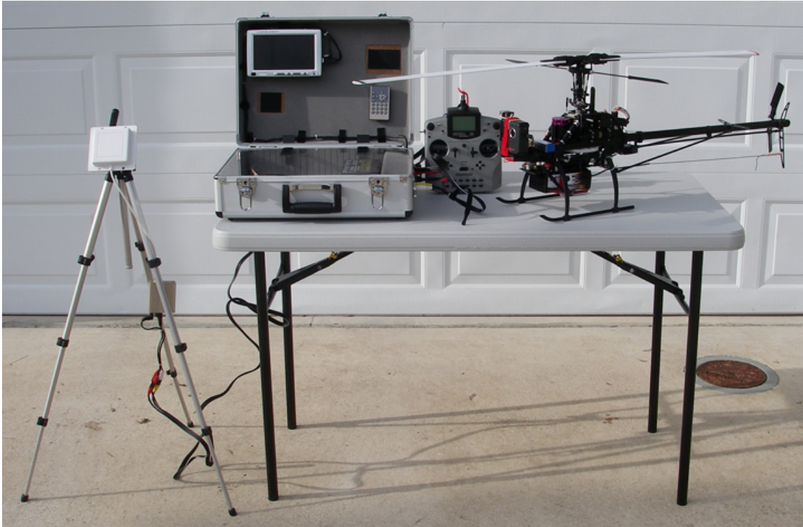
Figure 4-12 Century Helicopter, Swift 16 prepped for aerial photography. Included also is the base station, Multiplex transmitter, and the audio/video telemetry base station
