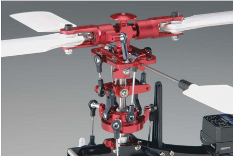
Figure 2-2 This is an example of the swash plate and rotor head control linkages.
