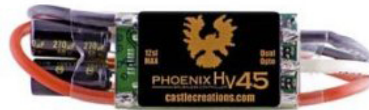
Figure 4-7 Castle Creation "Phoenix HV45 ESC" electronic speed controller.
