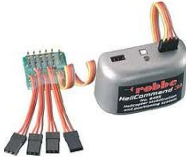
Figure 4-10 HeliCommand 3A Flight Augmentation Computer and Interface.
