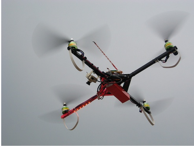
Figure 2-3 Quadcopter in flight, one of many variants of non-coaxial multi-rotor aircraft. © 2009, Stevens Institute of Technology
