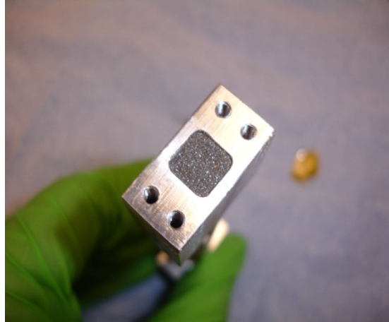
Figure 5: Filled particle dampener cavity of CP7 Test Beam.
