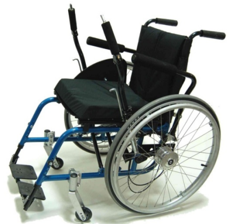
Figure 11. Rio Pivot Attachment with Rio Wheelchair iv
