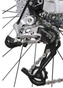
Figure 25. Standard Bicycle Rear Gearset with Derailleur. xi
