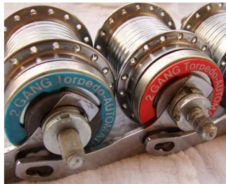
Figure 27. Examples of Automatic Shifting Hubs xiii
