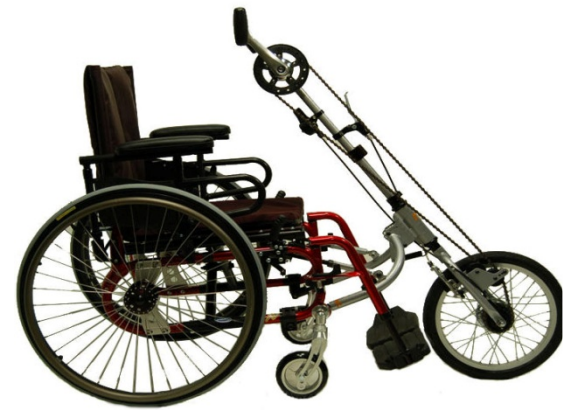
Figure 10. Rio Dragonfly Handcycle Attachment with Rio Wheelchair vii
