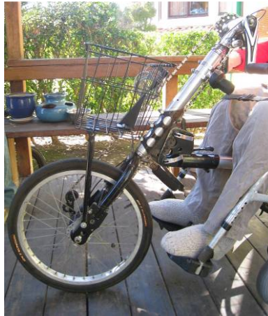
Figure 1. Greg O'Kelly's Current FWD Hand Cycle Attachment.
