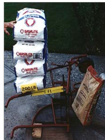
Figure 4. Backrest Tubes Inward Force
