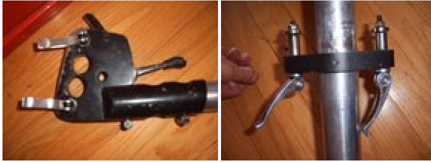
Figure 22. Quick-Release Mechanism from Mr. O'Kelly's Current Handcycle Attachment.
