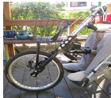
Figure 8. Modified Team Hybrid Coyote Attachment
