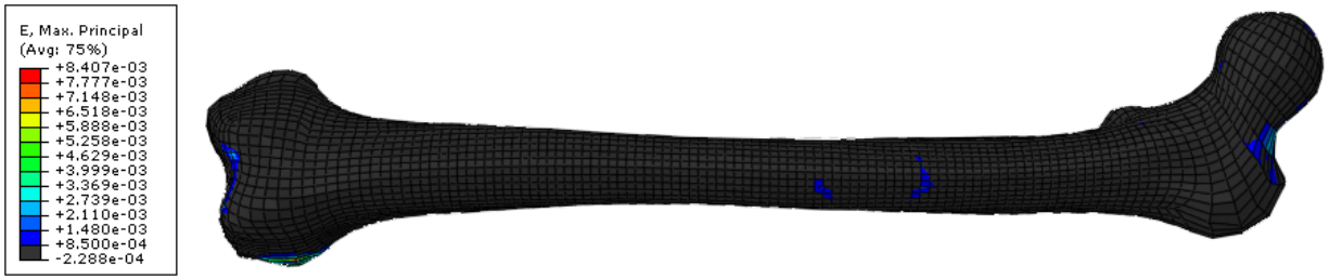
(a) SPRP strain distribution for a 105° single leg extension exercise.
