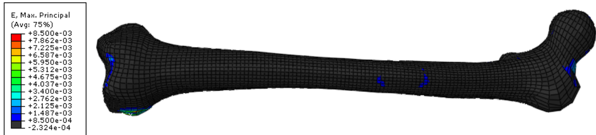
(b) SPNT strain distribution for a 105° single leg extension exercise.
