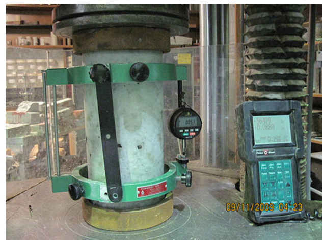
Fig. 5 Test set up for finding modulus of elasticity.
