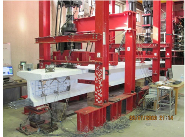
Fig. 4 Test set up for girders.
