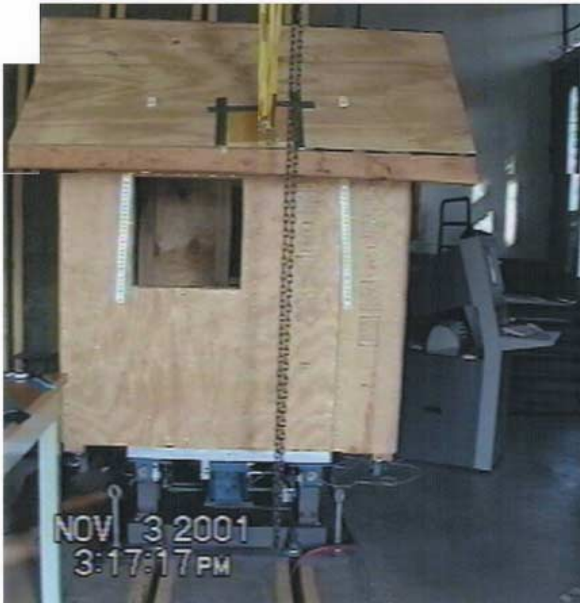
Figure 7 View of the Longitudinal Side with the Model Bolted onto Shake Table. The Workstation is Visible in the Background.
