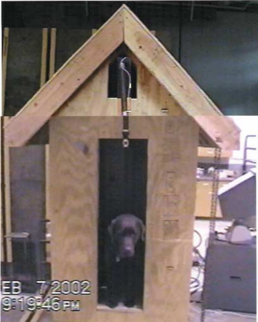
Figure 6 View of the Transverse Side with the Model Bolted onto Shake Table. The Model is plumbed with a Steel Sprinkler System
