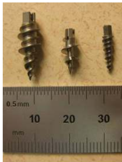
Figure 3-6: 6.5mm Smith & Nephew Twinfix (left), 5mm Mitek Fastin RC (middle), and 3.5mm Smith & Nephew Twinfix (right) suture anchors.
