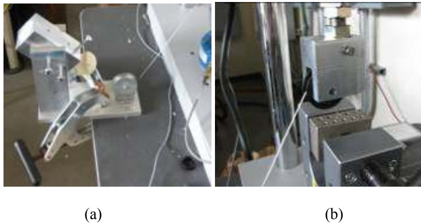
Figure 3-8: Experimental setup of potted humeral bone subassembly in bone holding fixture to investigate the effects of humeral bone elevation and suture anchor type on the pullout strength.
