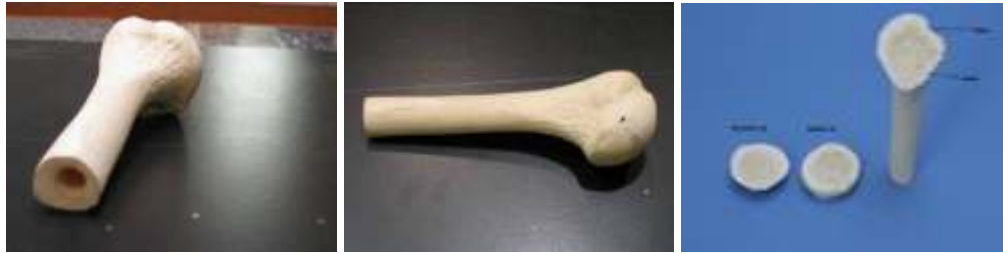
Figure 3-4: SAWBONES humeri with distal hole for placement onto potting base.
