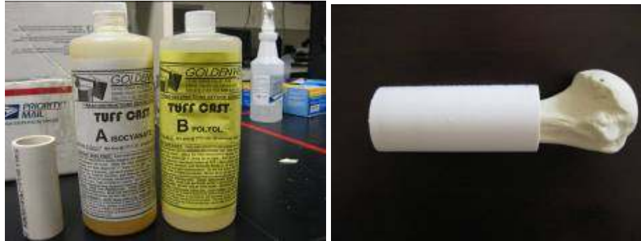
Figure 3-5: Isocyanate and Polyol solutions (left). Potted humerus subassembly (right).
