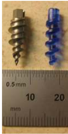
Figure 3-2: 6.5mm Smith & Nephew Twinfix (left) and 5mm Mitek Spiralok (right) suture anchors.
