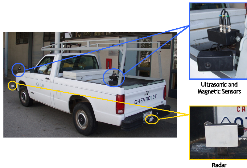
Figure 28. Test vehicle (pickup truck).
