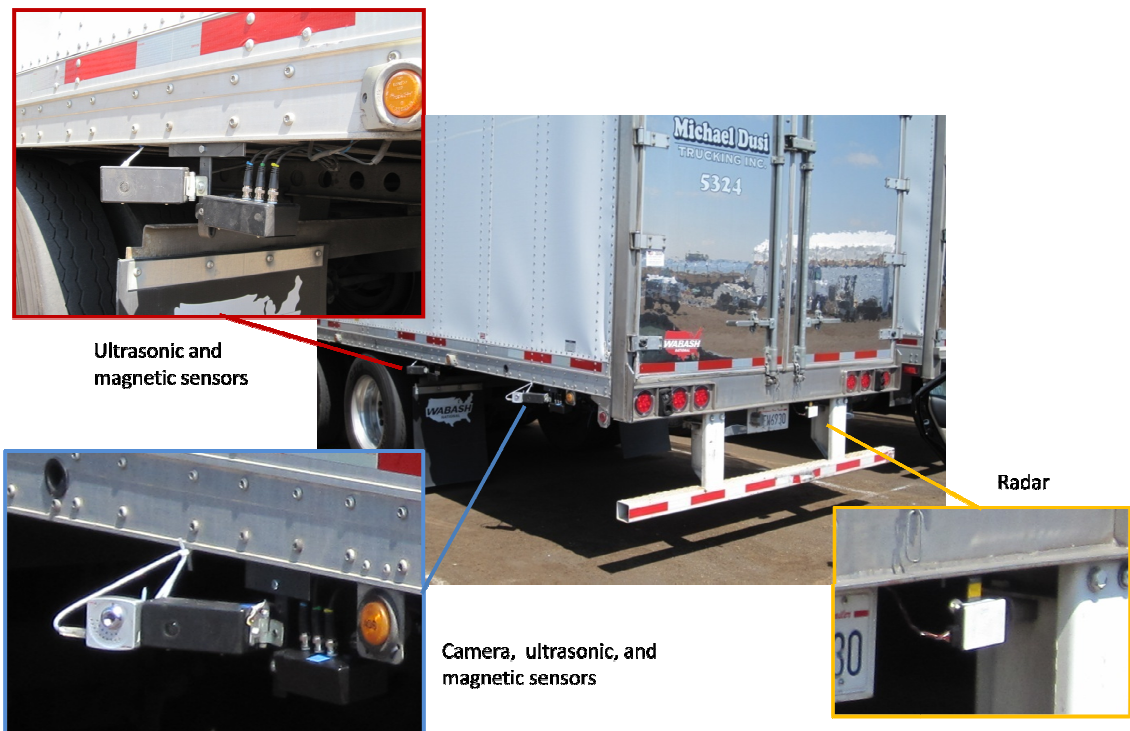
Figure 43. Sensor placement on large truck.
