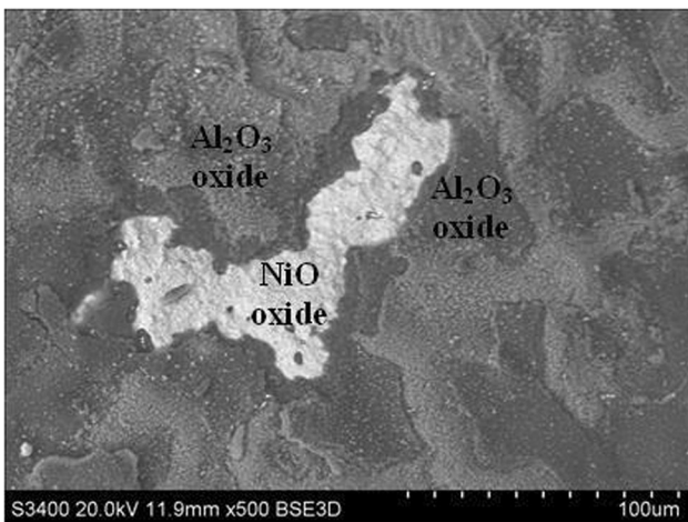
Fig. 17 SEM micrographs of oxides formed on the aluminide coating deposited by the CVD method after 30 cycles of oxidation at 1100^\circ\text{C} in the air atmosphere
