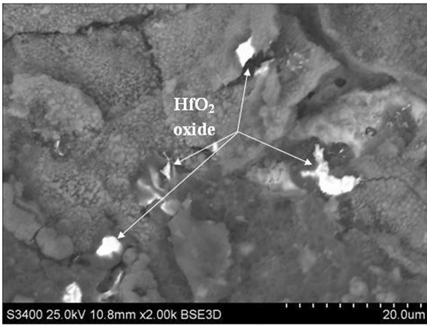
Fig. 11 SEM micrographs of the \text{Al}_2\text{O}_3 and \text{HfO}_2 oxides formed on the aluminide coating deposited by the VPA method after 10 cycles of oxidation at 1100 °C in the air atmosphere
