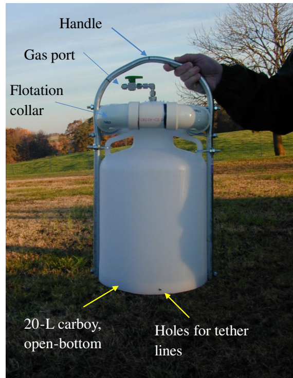
Fig. 1 Gas collectors constructed from open-bottom 20-L carboys. Graduations for evaluation of gas volumes located on the side of the carboy
