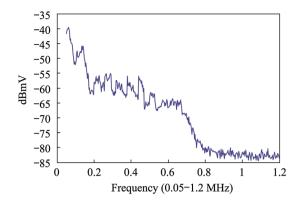
Fig. 1 The average value envelope spectrum of interferential voltage on device's power line while working normally
