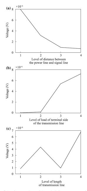
interference voltage of L-terminal for the three parameters at four levels is plotted in Fig. 5.
