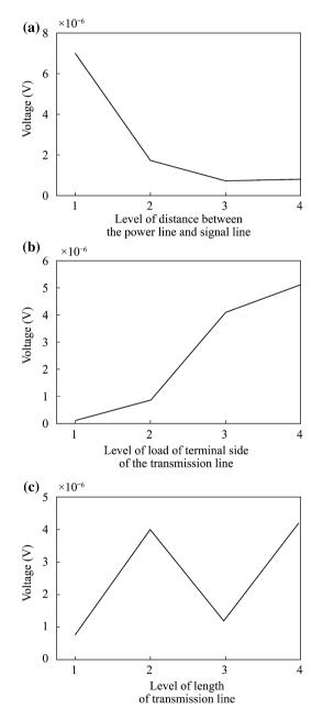
Fig. 4 Interference voltage of S-terminal for parameters at four levels. **a** Level of distance between the power line and signal line; **b** level of load of terminal side of the transmission line; **c** level of length of transmission line
