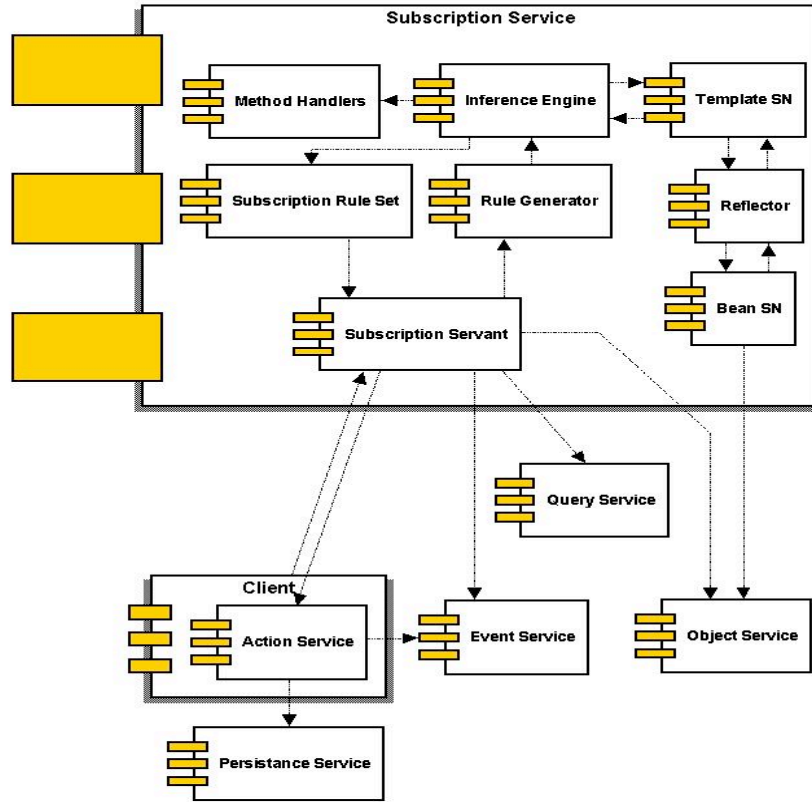
Fig.28: Inference engine-based subscription service architecture
