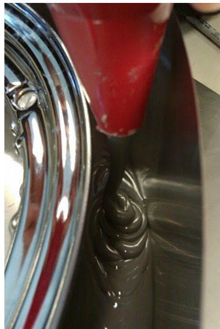
Figure 33: Detail of casting resin being poured. Resin is best worked with at warm temperatures as it has an extremely low viscosity.
