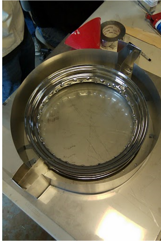
Figure 30: Rim placed in sheet metal hoop with parting line dividers.
