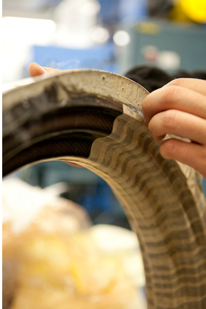
Figure 35: Hoop mold with carbon fiber Pre-preg laid in and Teflon strips being placed. The Teflon strips are the light tan seen in the right portion of the image.
