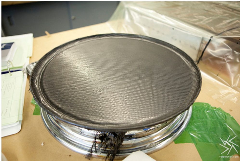
Figure 34: Completed center mold. Notice the scalloped profile around the edge which matches with the finished rim shape to create male and female surfaces for bonding.
