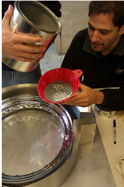
Figure 32: Pouring the casting resin into the mold for the mold.
