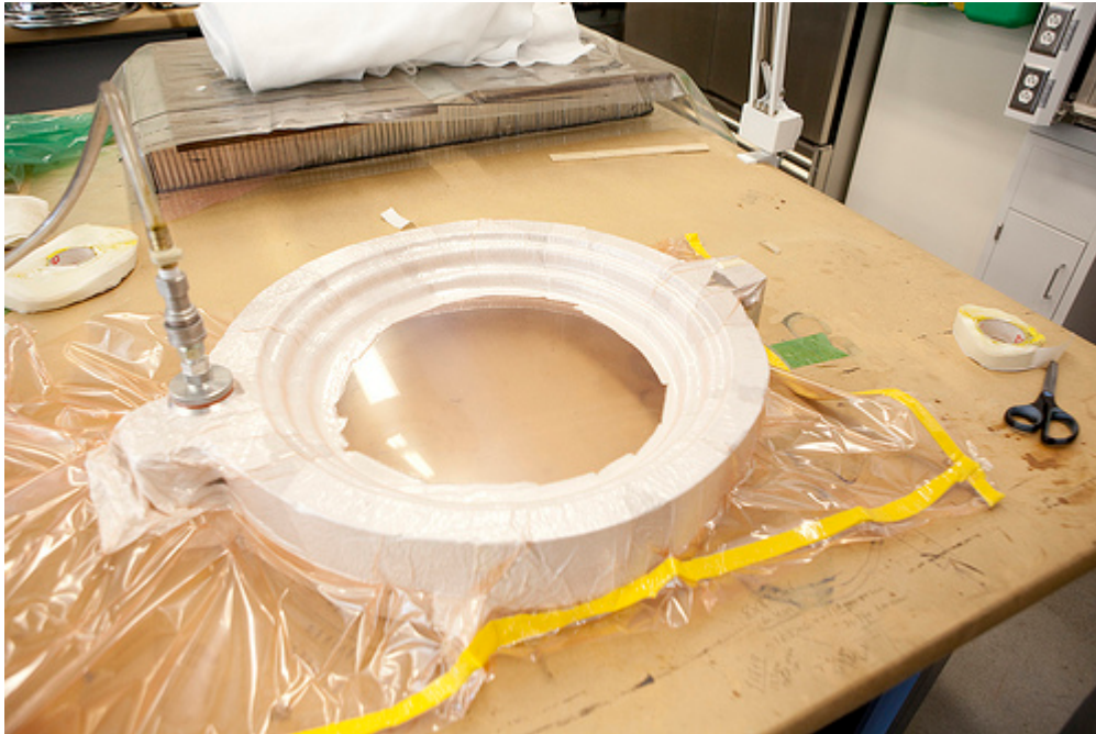
Figure 36: Mold placed in a vacuum bag. The vacuum bag material used was stretchy so that it would conform to the inner surface of the rim.
