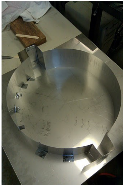
Figure 29: Concentric sheet metal hoop for mold construction.
