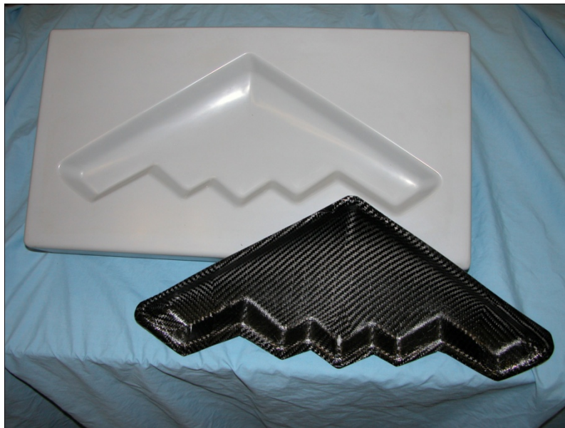
Figure 16: Female Composite Mold and Resulting Carbon Fiber Part (19)
