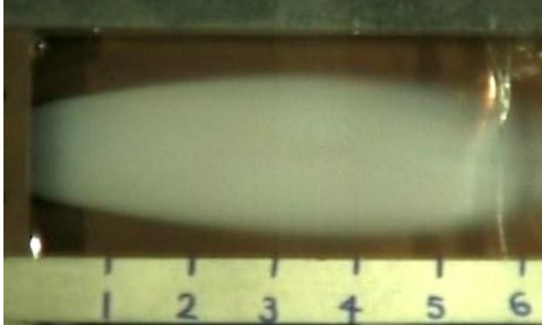
Figure 5-1 Nitrogen condensation plume in the mixing chamber at a pressure ratio of 95^4
