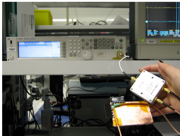
Figure 9b: Prototype set up to obtain a 90 degrees phase shift. Agilent N5181A MXG Analog Signal Generator (Frequency 400 – 413 MHz. Amplitude: 0.0 dBm).
