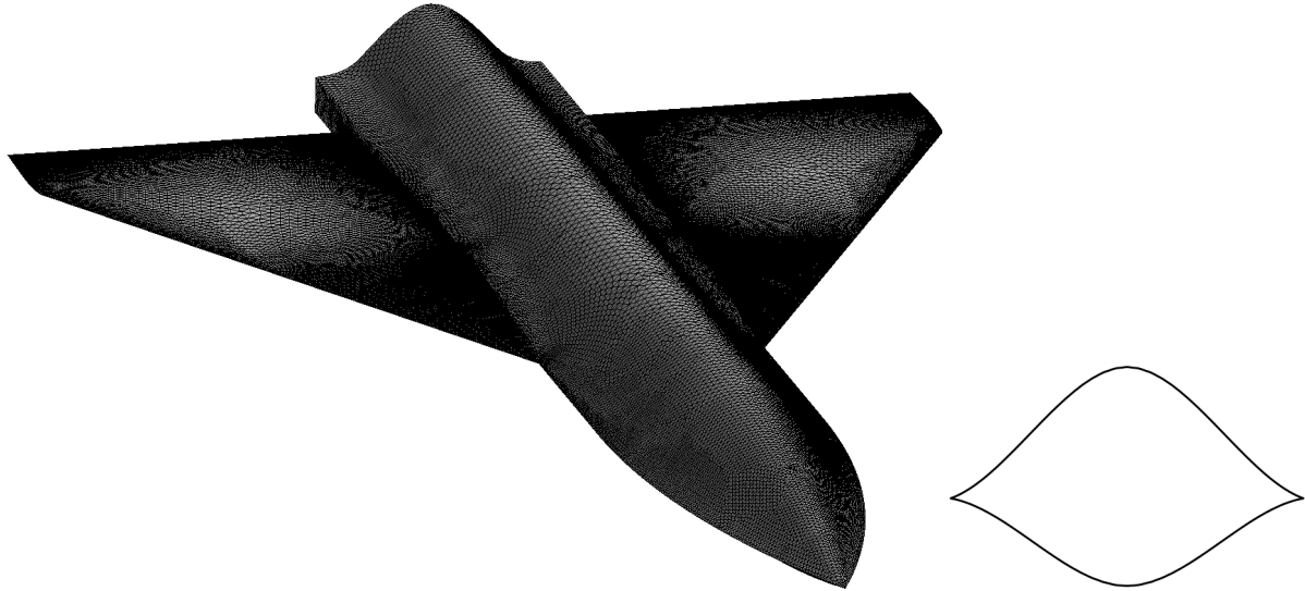
(a) Figure 1. (a) Schematic of overall MTVI configuration and surface mesh. (b) Schematic of forebody cross section with 30^\circ chine.
