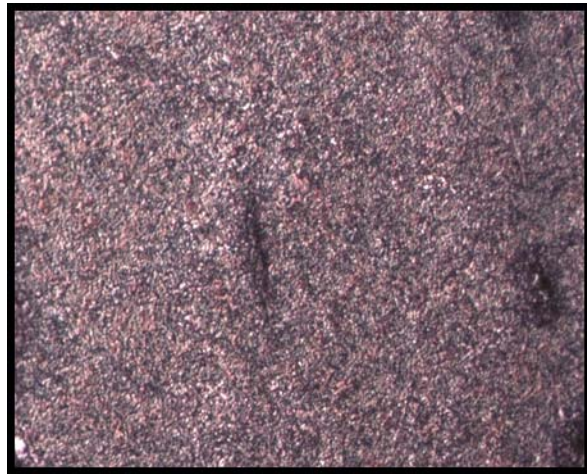
Figure 6.11 Barrel Samples 2.1 (a), 2.2 (b), and 2.3 (c) in a 2% Nital Solution at .75x
