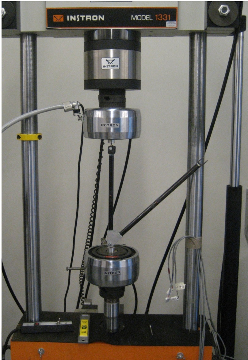
Figure 20: Lower A-arm on Instron Force Tester
