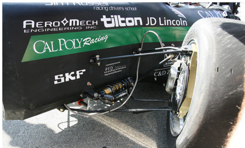
Figure 1: Broken Suspension Components
