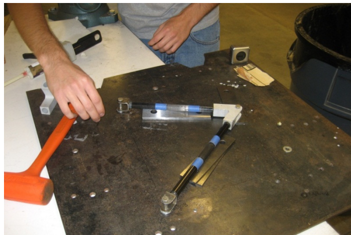
Figure 17: Bonded and Assembled Lower A-arm in Jig
