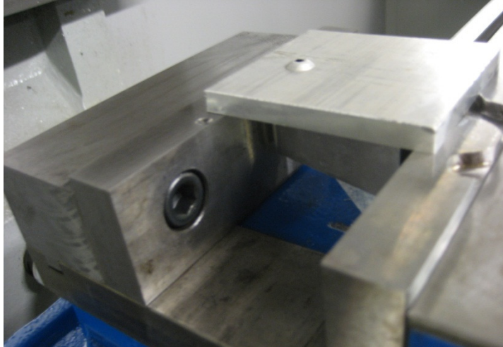
Figure 13: Second Setup for CNC Joint
