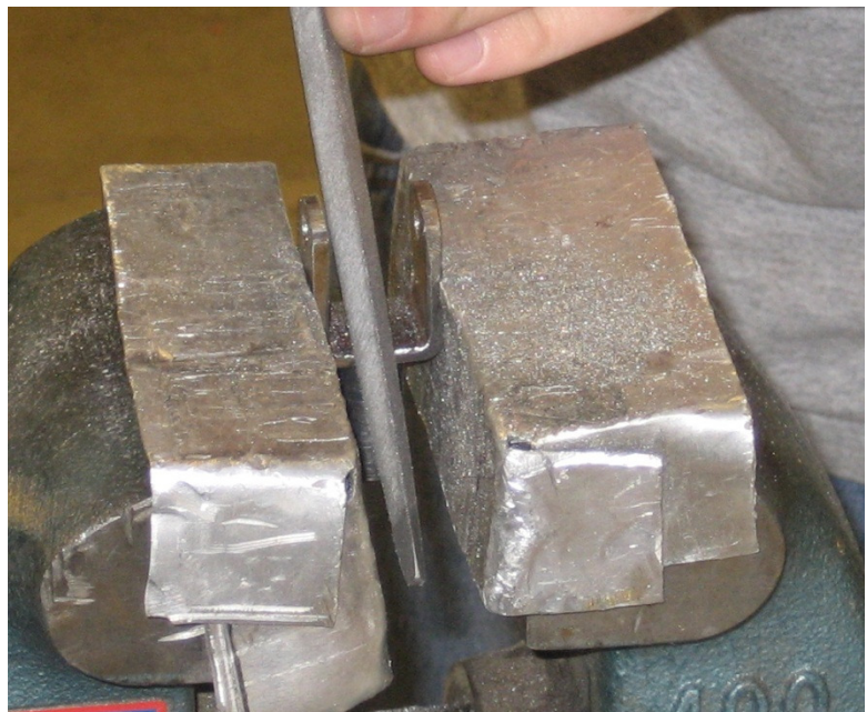
Figure 15: Final Preparation of Steel End Joint
