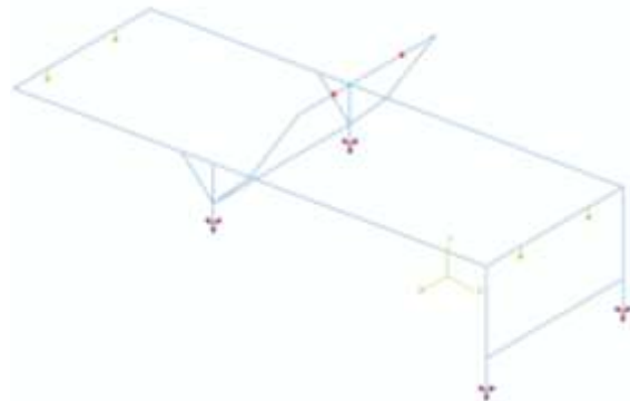
Figure 23D. Similar to load case B. Offset load on rear of frame and seat support. 150lbs down on right rear, 90lbs down on left rear, 40lbs down on footrest right, 10lbs down on footrest left.
