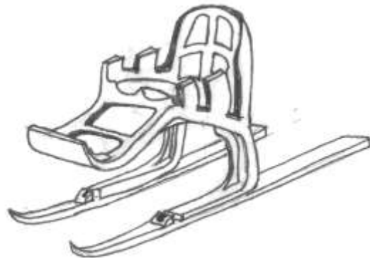
Figure 14. Carbon Fiber Uni-body concept design sketch. Frame and seat are built with one integrate carbon fiber design.
