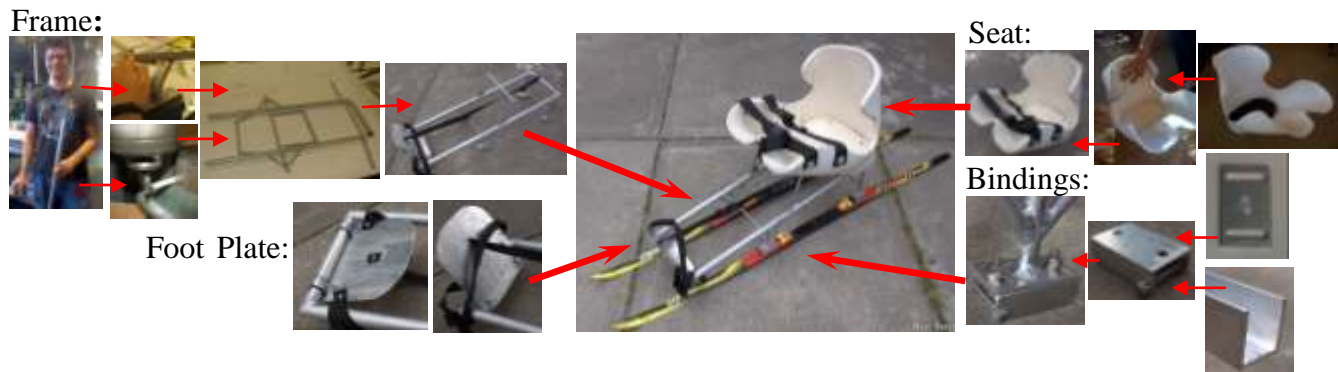
Figure 26. Diagram of the four main manufacturing tracks: the frame, seat, bindings and foot plate. The final assembly is shown in the middle.
