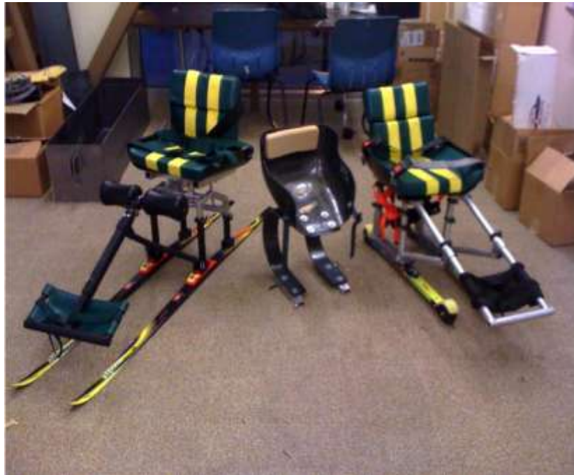
Figure 2. Cal Poly sit ski designs: Ski Lynx on the left carbon leaf spring design in the middle and the modular CP sit ski design on the right (equipped with roller skis for testing on pavement). (Barats)
