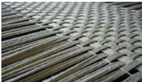
Figure 9. Hemp cloth composite that could be used for seat [H].
