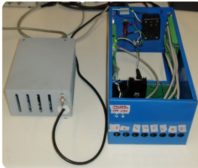
Figure 3.9: DAQ Interface with power supply.
