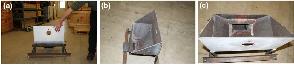
Figure 4. Photographs of the “birdhouse” attachment to the deflector plate on the bullet trap that allowed collecting and concentrating fragments onto plates painted with temperature sensitive paints.
