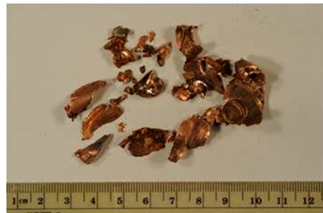
Figure 6. Photographs of bullet fragments collected after impact from water-filled collector tank.
