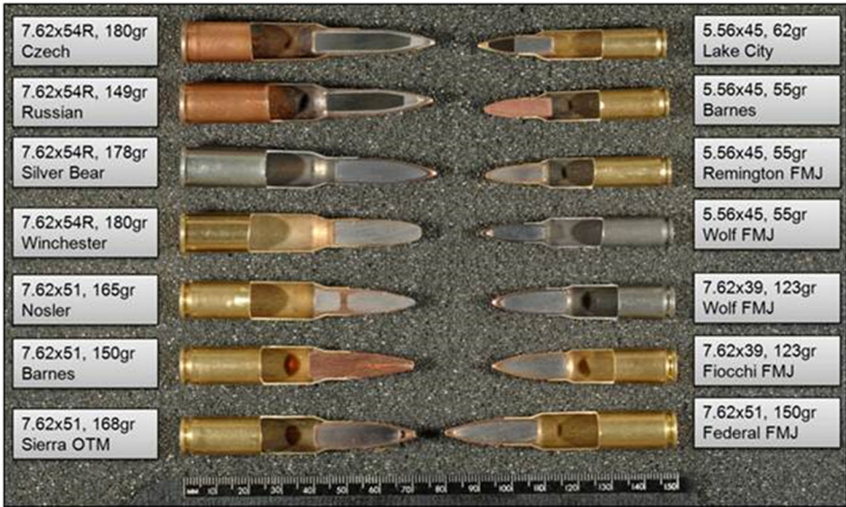
Figure 2. Cross-sections of bullets used in this study. Photograph by J. Kautz.
