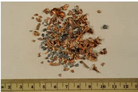
Figure 6. Photographs of bullet fragments collected after impact from water-filled collector tank.
