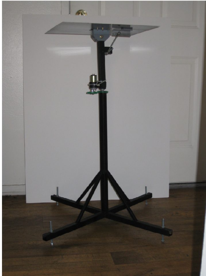
Figure 10: Support for Tracking Mechanisms
