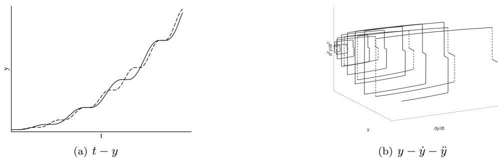
Figure 16. Displacement as a function of time and regressor space coverage for the integrated DC PWLS maneuver
