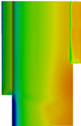
Figure 11. Surface pressures for part-span flap configuration.
