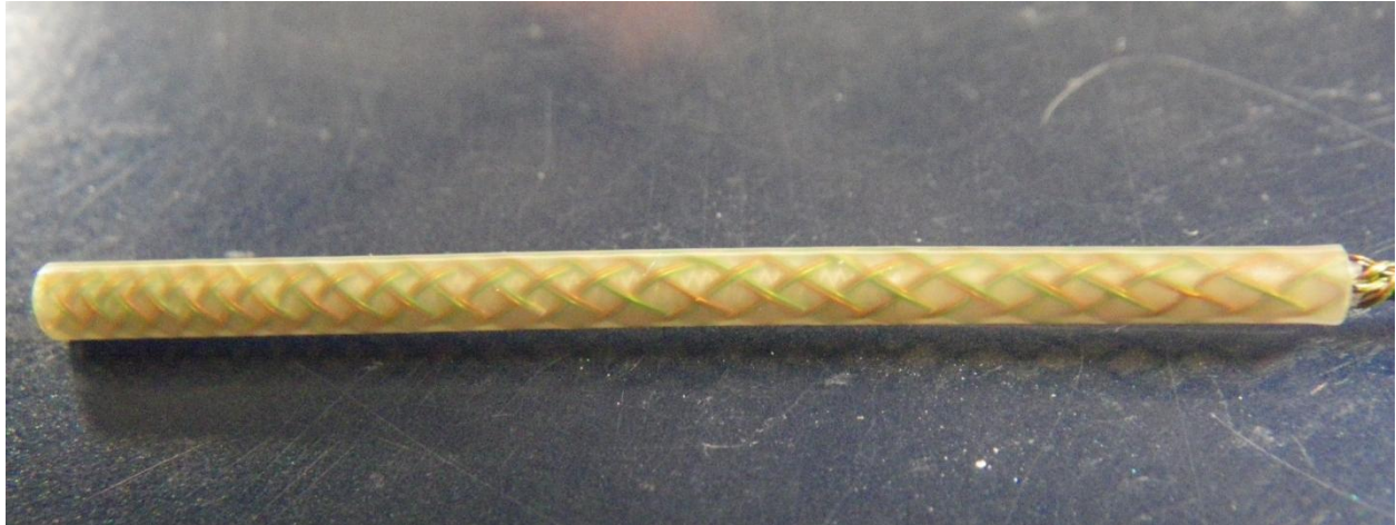
Figure 12: Change in braid density at proximal end of catheter. The variation in the braid density will affect the accuracy of the wire tracking GUI.
