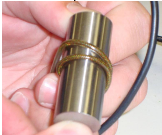
Figure 11: Catheter during steering compliance test. There are no sections of the catheter that have kinks as a result of wrapping around the test gage.
