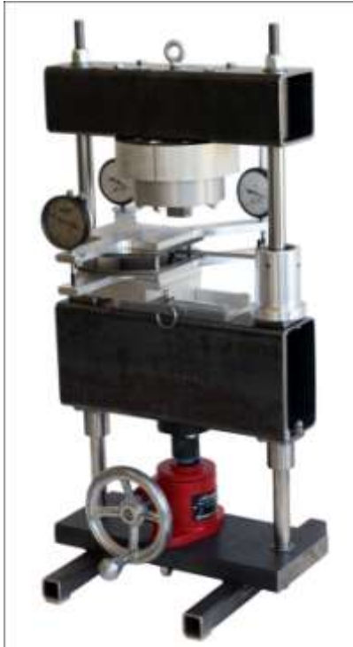
Figure 188. Final assembly of brinell limit test machine.
