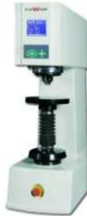
Figure 1. 3000 BLD Brinell Tester from Wilson Instruments.
