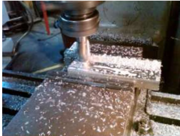
Figure 16. Milling of the track system
