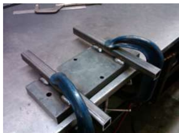
Figure 17. Dial indicator plate being machined on a CNC mill and base plate after welding.
