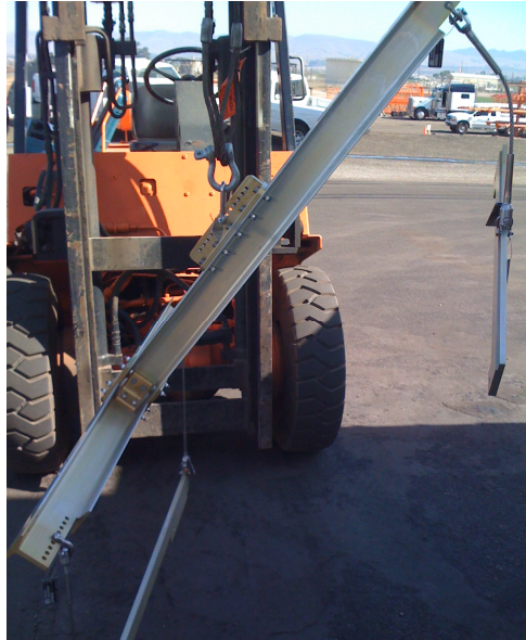
Figure 60. Unbalanced horizontal lift sling.
