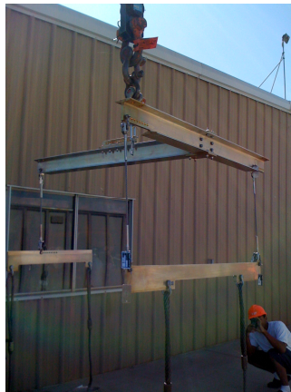
Figure 63. Proof test attachment points.
