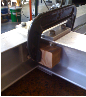
Figure 37. I-beam assembly clamped in place.
