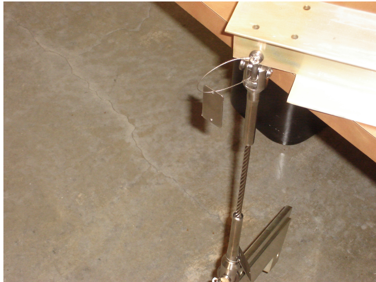
Fig 26. Rear Cable Assembly Before NDI Testing
