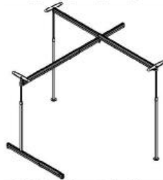
Figure 11. Three point lift sling.
