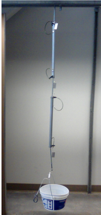
Fig 81. Proof test setup for part 20005, cover support assembly.
