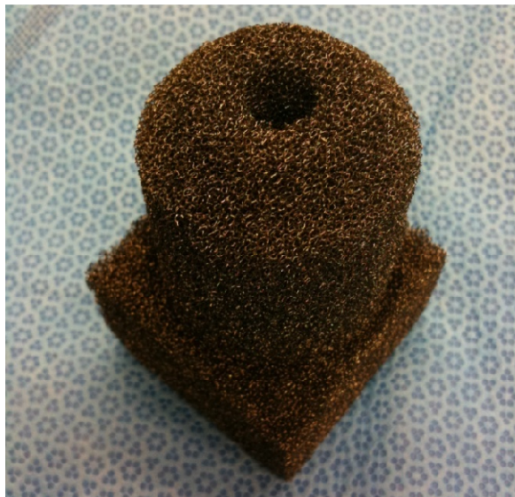
Figure 11. Carbon foam after being reamed to the shape of the prepared femoral head
