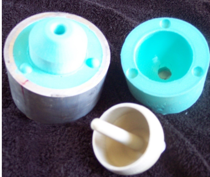
Figure 9. Two part silicone molds were used to create plastic models of femoral resurfacing components.
