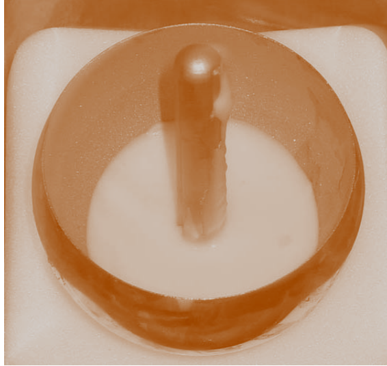
Figure 12. A demonstration of an implant model being filled with PMMA to 50% of its depth
