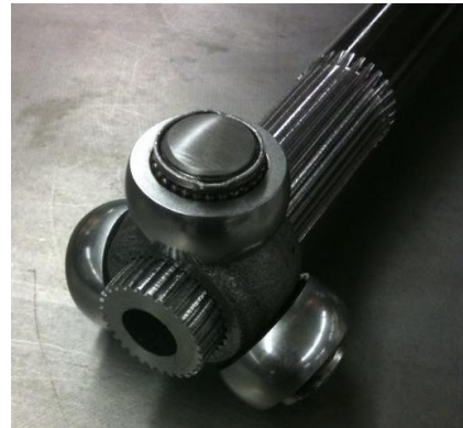
Figure 5.12: Spined half-shaft with tri-pod bearing
