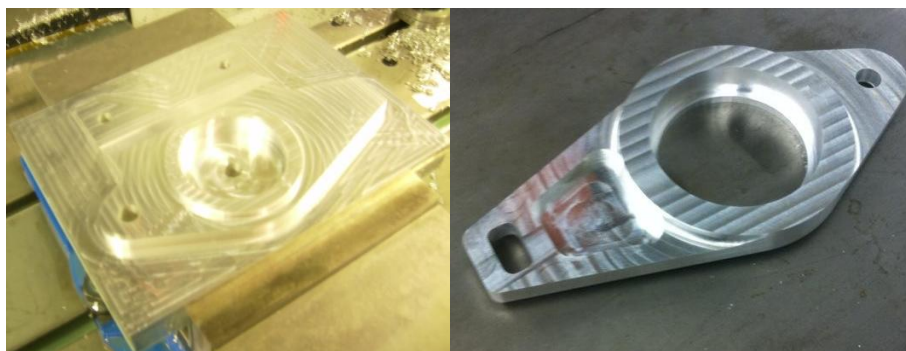
Figure 5.11: Left- Brake side differential upright after first side of machining. Right- Sprocket side differential upright fully machined.
