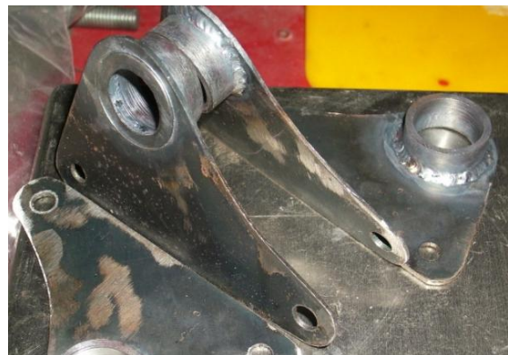
Figure 5.3: Rockers after welding of bearing cups
