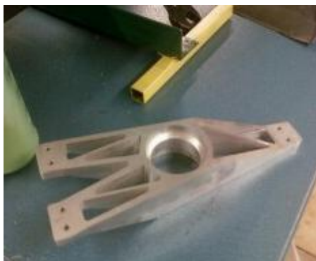
Figure 5.15: Upright right after machining process
