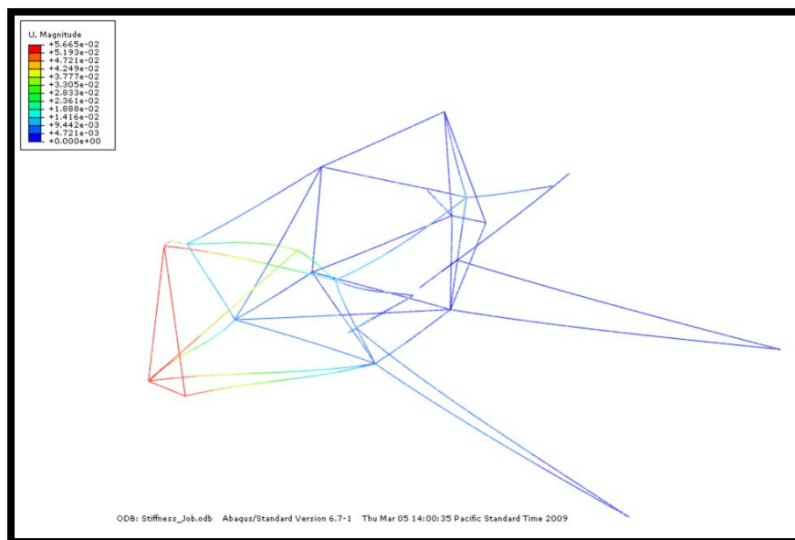
Figure 4.11: Chassis stiffness simulation of rear frame
