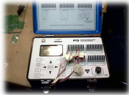
Figure 6.6: Full Wheatstone bridge wired into P3 data acquisition box.
