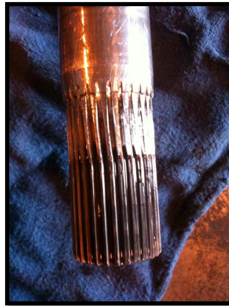
Figure 6.11: Result of torsional twist on brake side (left) axle stub
