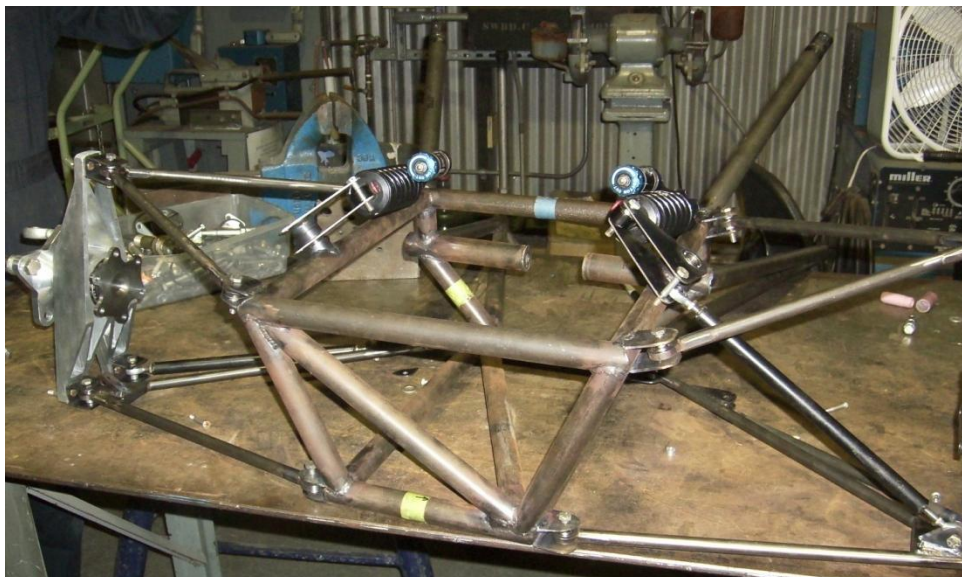
Figure 5.8: Rear frame completely welded and assembled with the suspension components
