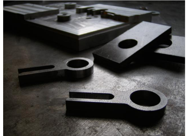
Figure 5.1: A-Arm wafer jig, blanks, and finished single wafers
