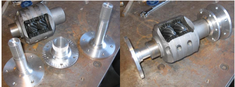
Figure 5.10: Differential axial stubs and sprocket insert completed and assembled in differential
