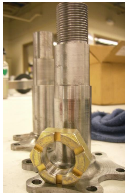
Figure 5.16: Final Steel Spindles and castle nut showing thread and sinusoidal spline.
