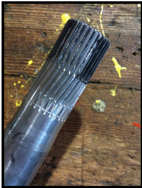
Figure 6.10: Results of torsional twist on sprocket side (right) axle stub
