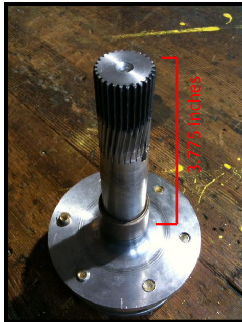
Figure 6.12: Length of twist is 3.775 inches
