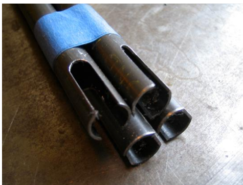
Figure 5.2: Notched A-Arm tubing
