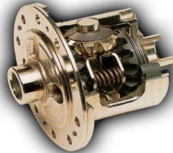
Figure 3.7: Representation of a limited slip clutch differential
