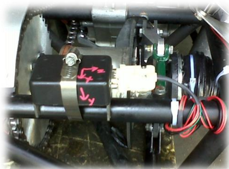
Figure 6.7: Accelerometer mounted on rear frame. This location proved to be vibration prone, so it was later relocated to a more dampened location on the monocoque.
