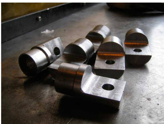
Figure 5.7: Single shear chassis bungs for upper frame mounts
