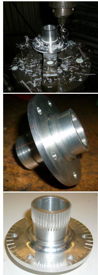
Figure 5.9: Top- drilling of Sprocket bolt holes. Middle-Bearing surface after sleeve was pressed on. Bottom- final part after splining
