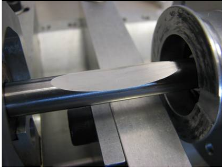
Figure 28: Precision ground flat in shaft to produce asymmetric stiffness
