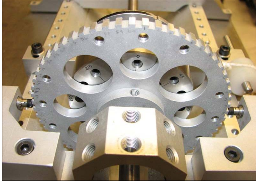
Figure 31: Torsional transducer consisting of a gear wheel and two proximity probes
