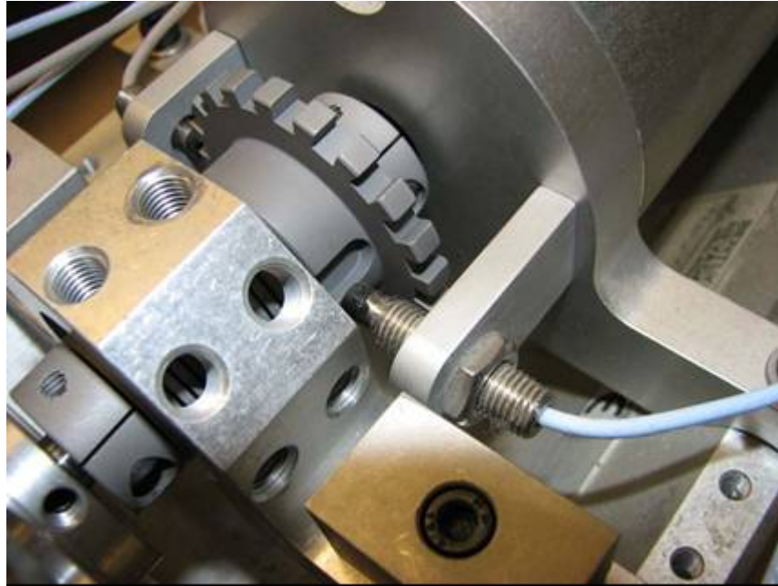
Figure 29: Reluctor wheel for motor speed control
