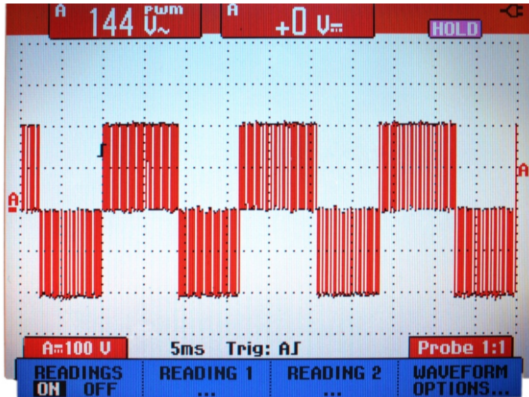
Figure 6-2 - Output Voltage at 2 kHz Switching Frequency (5ms/div)
