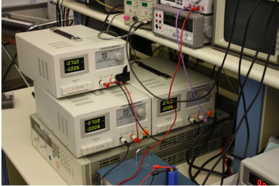
Figure 5-5 - Input Voltage Source
