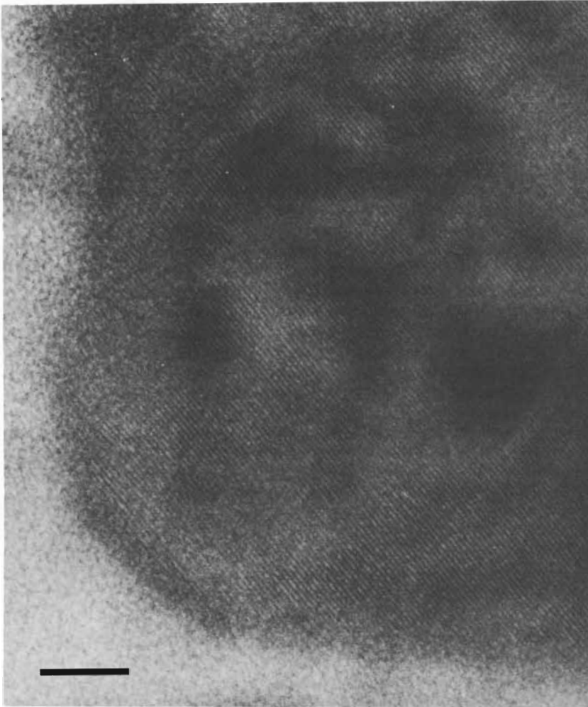
Figure 7. Lattice image showing (111) ( 3.13 \text{ \AA} ) fringes of \text{FeS}_2 . The fringes are coherent across the intracellular particle. Some discontinuities can be observed in the fringes but the images are coherent across these areas. These features reflect marked differences in particle thickness due to irregular crystal surfaces. Bar = 5.5 nm.
