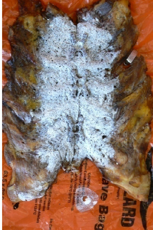
Figure 5.3: The cadaveric sternum must be coated with a special high-contrast "speckle" to record an acceptable amount of data.
