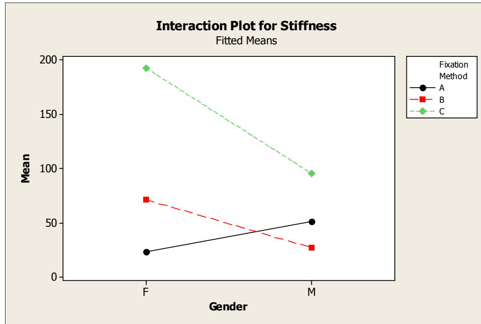
Figure 6.36: Interaction plot describing the effect of gender on each construct in regards stiffness tested in transverse shear.
