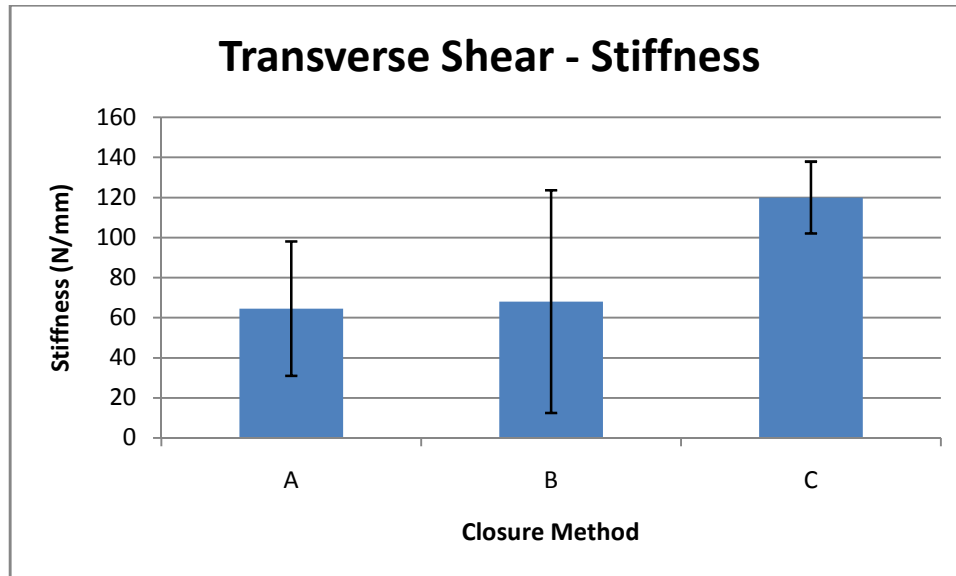
Figure 6.33: Rigidity (stiffness) of the various fixation methods tested in transverse shear. Columns denote mean values. Stiffness is measured in newtons of force per millimeter displacement. Error bars indicate one standard deviation.
