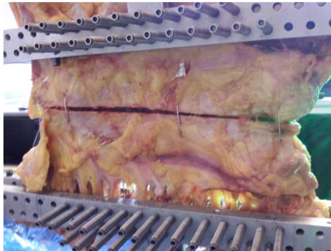
Figure 7.1: Picture taken at maximum displacement in the lateral distraction direction. Separation can be observed at the midline and rib fractures can be seen along the bottom clamp.
