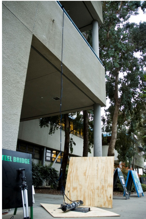
Figure 43. A legform was dropped from a 20 ft tall balcony onto a test section of SEA on the ground below.
