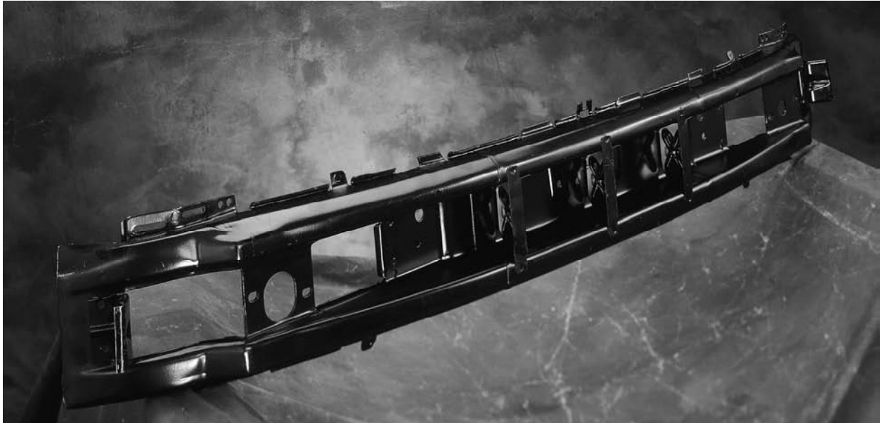
Figure 2. The Volkswagen Jetta (1993) has a hot stamped bumper beam [6].
