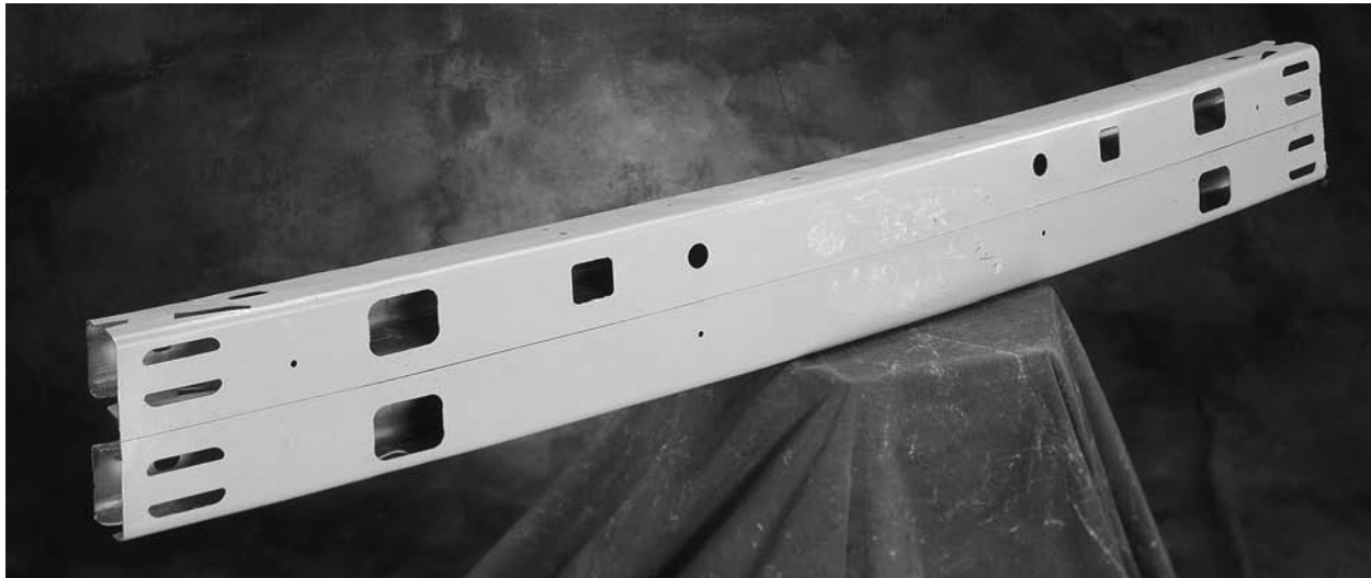
Figure 4. The Ford Taurus/Mercury Sable (1995) has a roll formed bumper beam [6].
