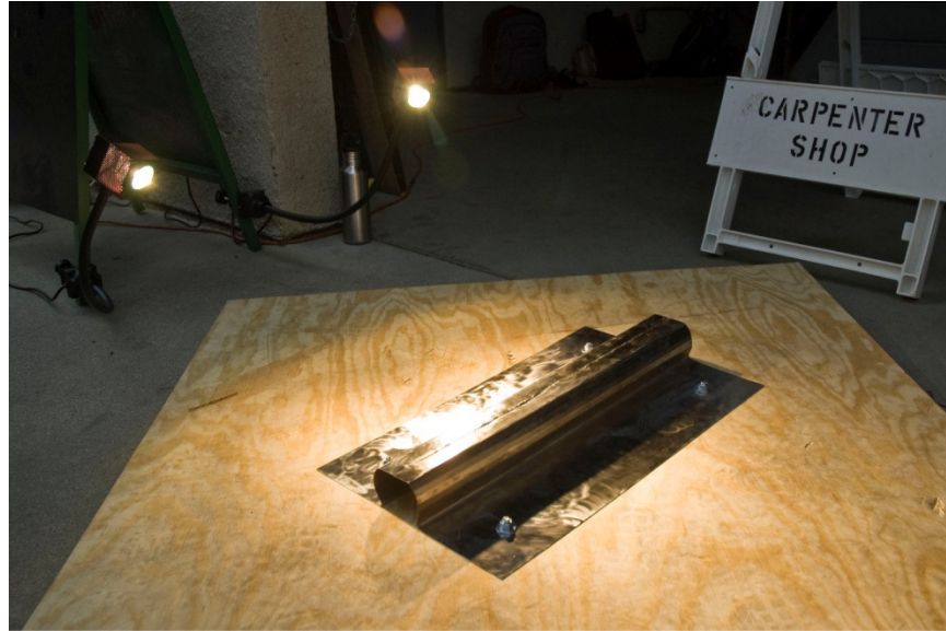
Figure 44. A test section of SEA was bolted onto a plywood test platform and placed beneath a balcony for the legform to be dropped on it.
