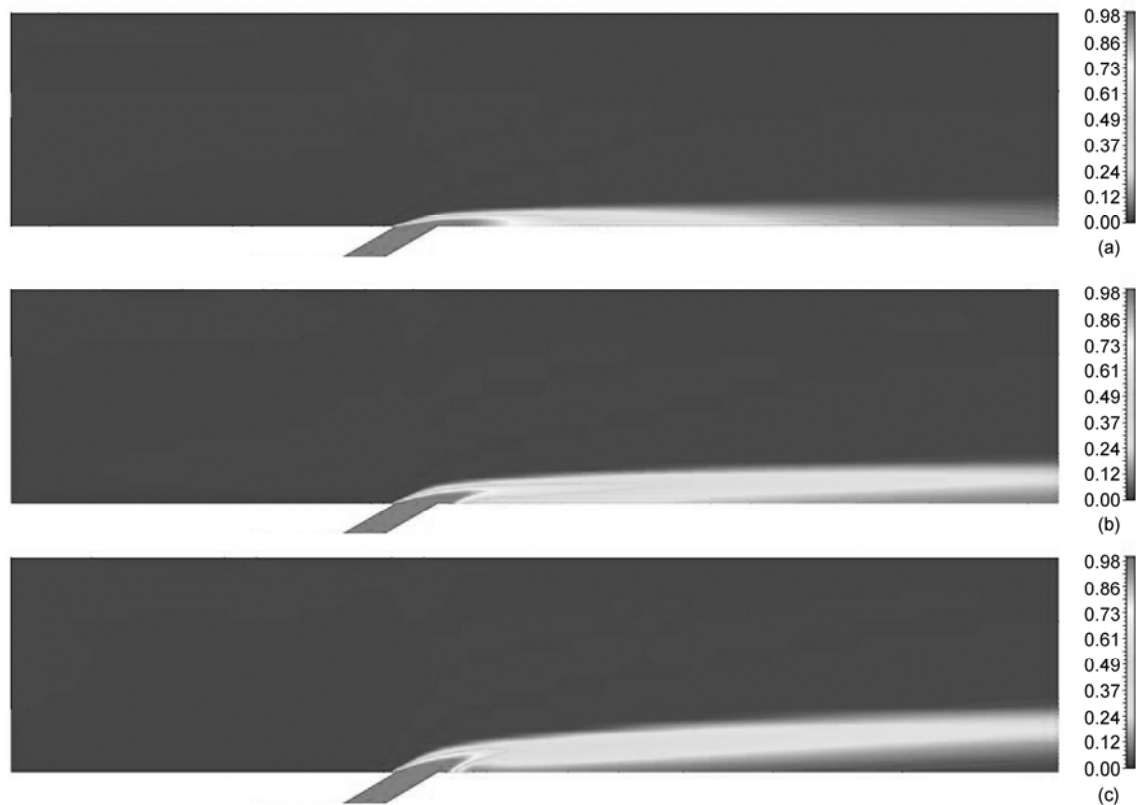
Figure 10 Mass fraction of \text{NH}_3 on the X-Z plane at different blowing ratios. (a) M = 0.5 ; (b) M = 1.0 ; (c) M = 1.5 .
