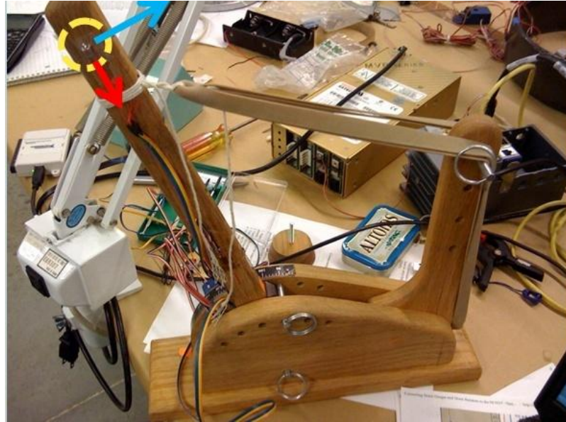
Figure 19. Catapult with accelerometer. The accelerometer is highlighted in yellow. The blue and red arrows represent the directions of tangential and normal acceleration, respectively.
