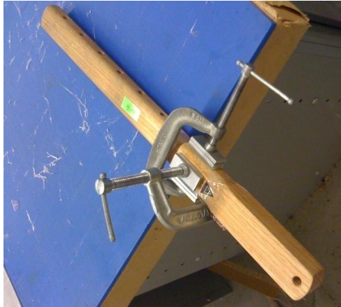
Figure 29. Strain gages curing under pressure from c-clamps.
