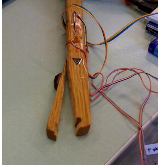
Figure 18. Broken catapult arm after some initial trials with two rubber bands.
