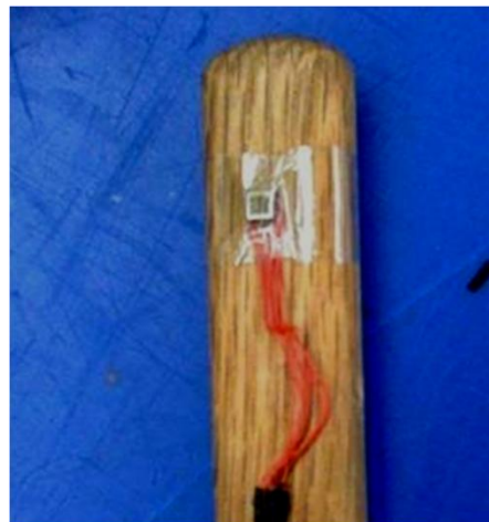
Figure 20. Close-up of accelerometer on catapult arm.
