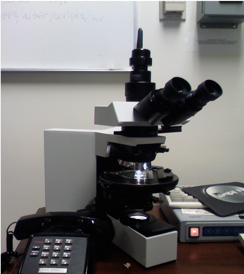
Figure 3.1 Olympus (Tokyo, Japan) microscope used in accordance with polarized light, in order to determine osteons types within each bone chip.
