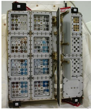
Fig. 40 EXPOSE-E integrated on the EuTEF platform before launch (Credit: ESA). The bottom two compartments and the lower half of next compartments contained the sample carriers (explosion drawing on the right, adapted, credit: Kayser-Threde) with the sample from ADAPT. Left vertical row is tray 1, open to space; middle vertical row is tray 2 with Mars conditions
