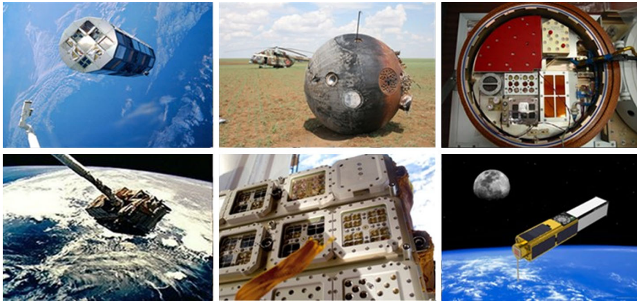
Fig. 7 Some of the past and current astrobiology devices used in Low Earth Orbit. From upper left to bottom right : LDEF, FOTON with embedded samples in its heat shield for STONE experiments, one lid of Biopan, EURECA, EXPOSE-R, and O/OREOS nanosatellite (artist's impression). (Credits: NASA, ROSCOSMOS, ESA/Kayser-Threde, NASA, ESA & NASA)
