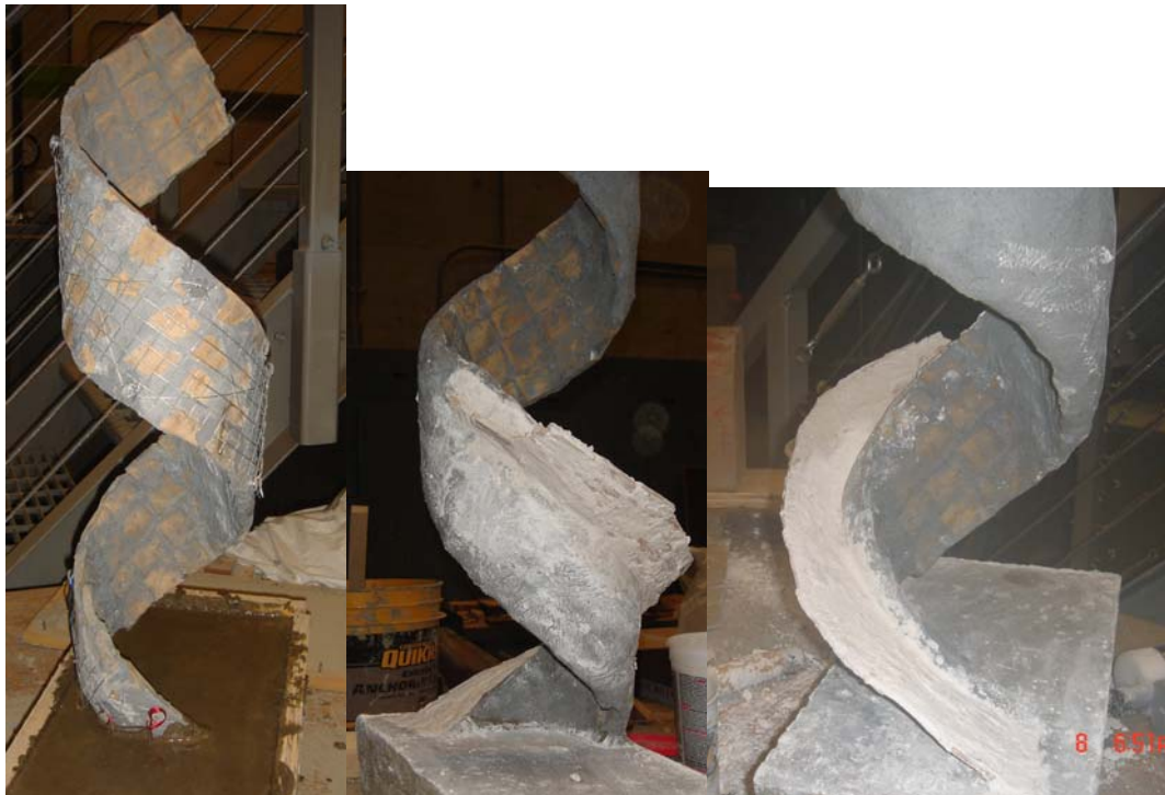
Figure 4. Benchtop Scale Spiral Staircase Made of Composite
