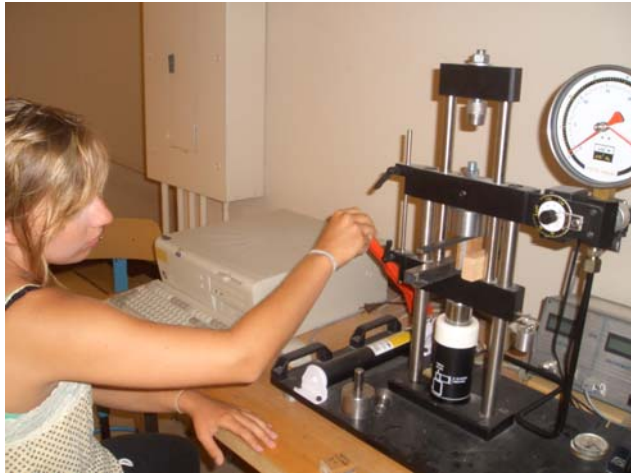
Figure 1. Shear Testing of Composite
